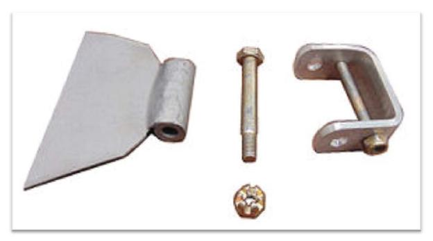
The pivot bolt (center) is an AN4-21 and the clamp bolt is an AN3-21.
